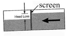
Figure 3: Head loss illustration: source: Butler K et all
