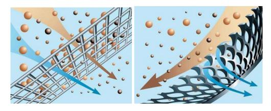
Figure 2: Illustration of direct (left) and indirect (right) screening: source CDS technologies
