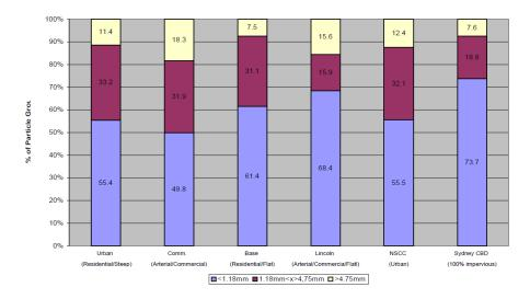
Figure 1: Particle size Characteristics of gross Pollutants
