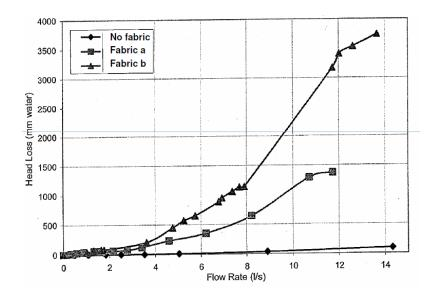
Figure 4: Difference in head loss between two screens with different aperture size source: Butler K et all
