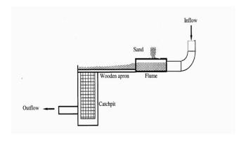
Figure 7: Laboratory Performance Testing Set up
