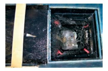
This is the suggested maintenance depth of the sump with a LittaTrap installed. The flow rate through the system was gradually increased over the test to a maximum of 15.6 l/sec. The average released concentration was 7.8-mg/l.
