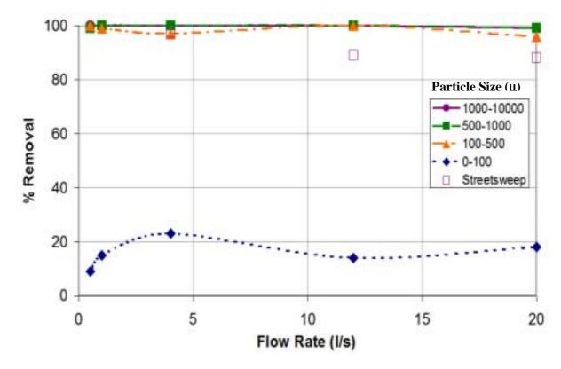
Figure 6 - Sediment Removal by the Catchpit Containing a Flogard CFS with a 400 µm mesh
