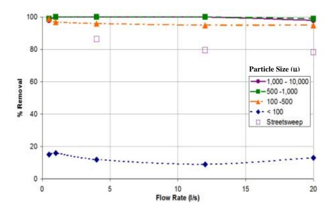
Figure 4 above shows the results in the standard catchpit without a CFS installed. Sediments larger than  $500\mu$  were completely removed for flows up to 20 l/s. The removal of  $100-500\mu$  particles decreases from 75% to 47% by increasing the flow from 0.5 l/s to 20 l/s, and only 18% of particles smaller than  $100\mu$  are trapped by the catchpit. Approximately 58% of the sediment collected from street sweepings were removed at 4 l/s.
