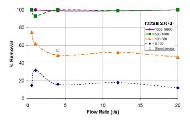
Figure 5 - Sediment Removal by the Catchpit Containing an Enviropod CFS with a 200 µm mesh
