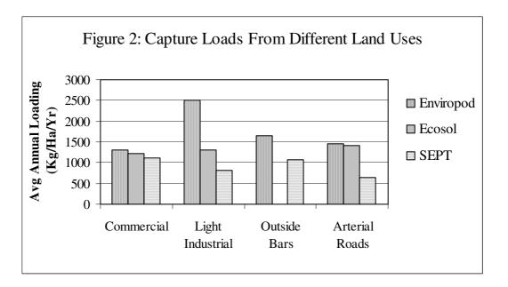
Enviropods and Ecosols collected higher capture loads for all land use types than the SEPTs. Capture loads were comparable for all three types of traps in Commercial Areas, including Salamanca Place. Enviropods and Ecosols captured less material in this area reflecting that stormwater pollution in Salamanca Place was not as significant as in other areas of the catchment.
