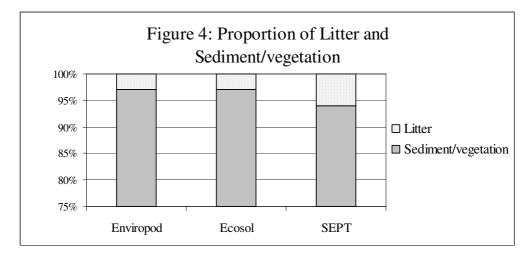
The proportion of litter to sediment/vegetation (by weight) varied between the SEPTs and the two other types of traps. Figure 4 above shows the percentage of litter and sediment/vegetation retained for each of the different types of traps.
