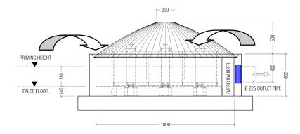
Figure 2: 6 Cartridge Low Drop StormFilter with Surface Entry (Elevation)
