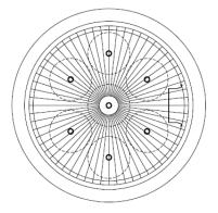
Figure 3: 6 Cartridge Low-Drop StormFilter with Surface Entry (Plan)
