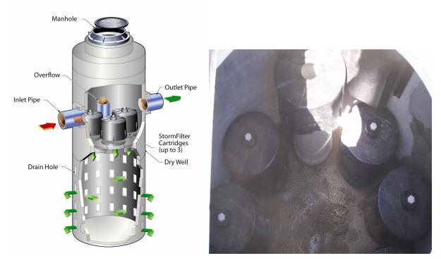
Figure 14: Conceptual perspective of soak well and inside the unit installed at Pound Road
