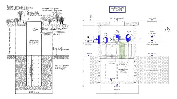
Figure 12: Christchurch City Deep Soakage Standard Detail and Modified Soakage Well StormFilter
