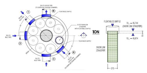
Figure 13: Soakage Well and Overflow with Floatables Baffle
