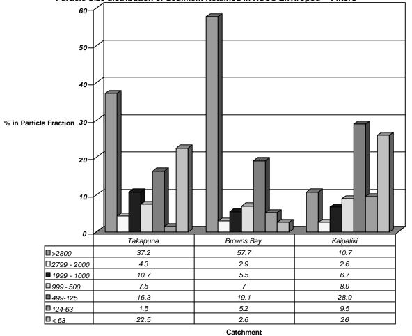
Particle Size distribution of Sediment Retained in NSCC Enviropod<sup>™</sup> Filters
