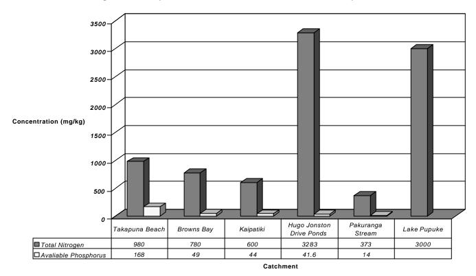
Nitrogen and Phosphorus in Retained sediments from NSCC Enviropod Filters
