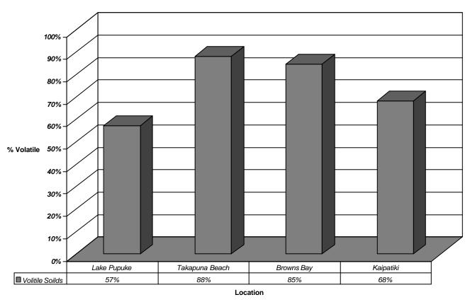
Volatile Solids in Sediment retained in NSCC EnviropodTM Filters
