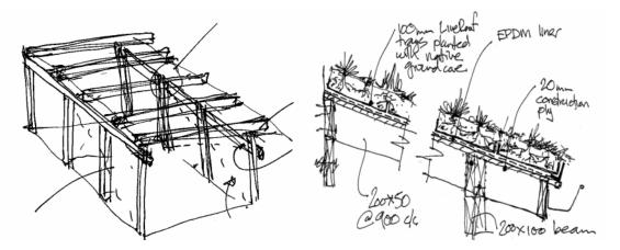
Figure 6: Carport and Live Roof Detail.
