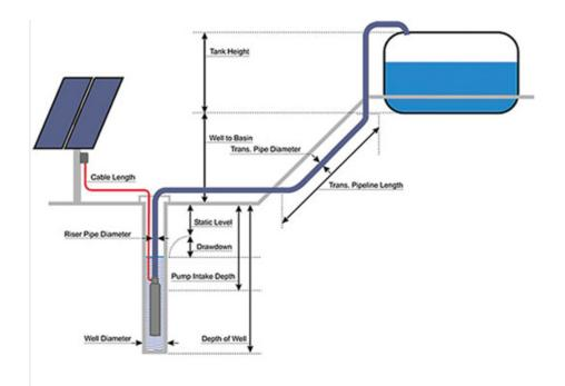
Figure 4: Solar Pumping System Schematic
