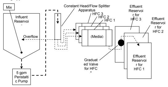
Figure 8: Schematic Laboratory Testing Apparatus
