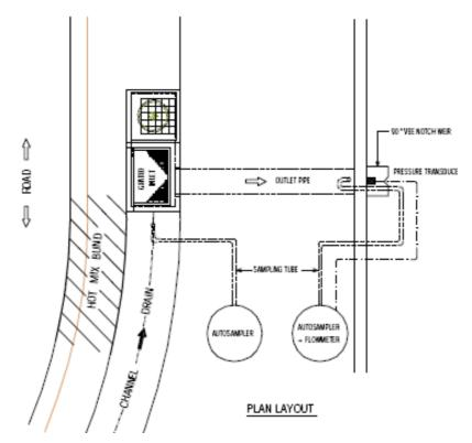
Figure 13: Field Trial Apparatus
