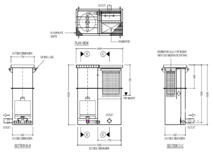
Figure 6: Construction Drawing of The SFEP Treatment Train
