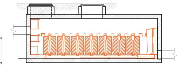
0.55m from inlet to outlet for low drop configurations, 0.7m for 46cm cartridges and 0.93m for 69cm cartridges
