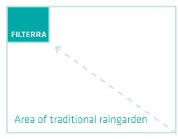
Based on a catchment area of  $2000m^2$  in Auckland, a 2% rain garden is at least  $50m^2$ . The Filterra® required to treat all flows is  $8.4m^2$ :  $4m \times 2.1m$
