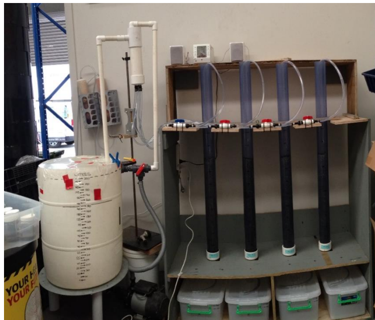
Figure 3 Photo of the four column test setup
