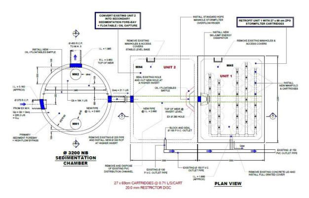
Figure 5: Retrofit (StormFilter) Layout Plan (Source: Stormwater360) Water New Zealand's 2017 Stormwater Conference
