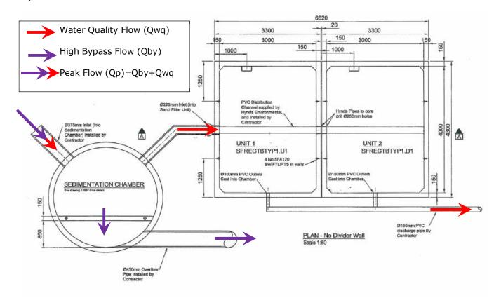
Figure 2: Original Sandfilter Layout Plan (Amended from Source: Hynds Environmental)
