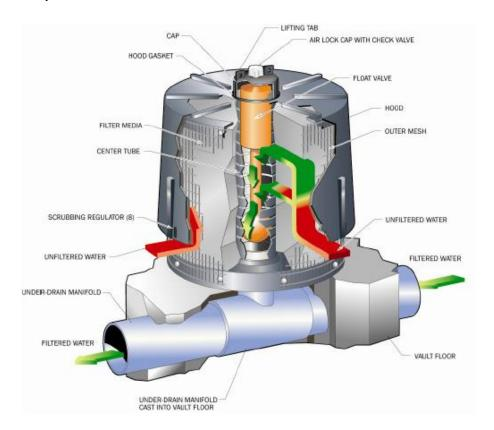
Figure 4: StormFilter Cartridge
