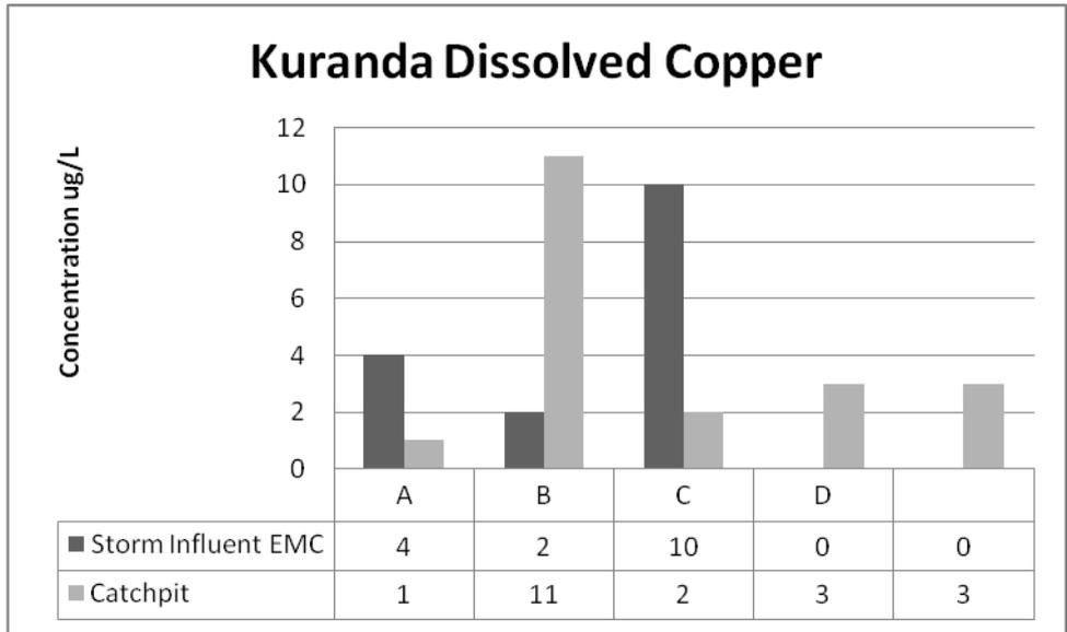
**Fig 4. Kuranda SFEP: Dissolved copper concentrations**
