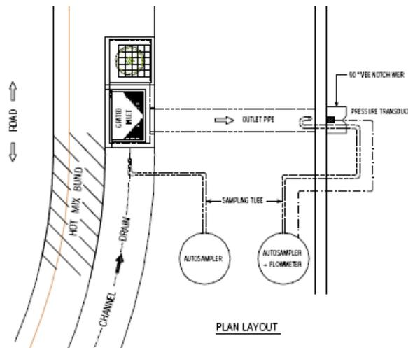
**Fig 2. Kuranda SFEP: Experimental set-up**
