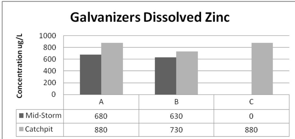
**Fig 7. Galvanizing Facility Dissolved Zinc Concentrations**
