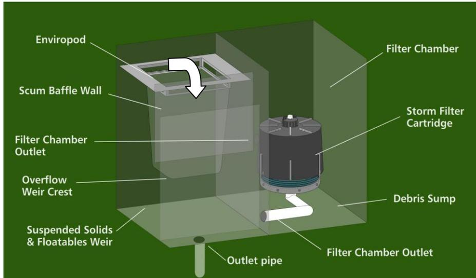
**Fig 1. Kuranda SFEP: Treatment train layout.**
