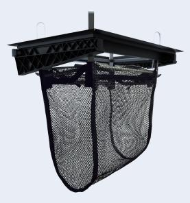
**The LittaTrap**<sup>™</sup> is a storm drain insert system. It is readily installed in new or existing storm drains and may be configured to capture a variety of pollutants. The LittaTrap<sup>™</sup> is hand maintainable, allowing for low cost and frequent maintenance.
