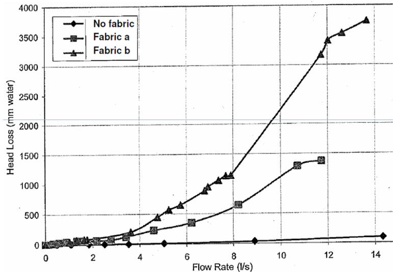
Figure 4: Difference in head loss between two screens with different aperture size
